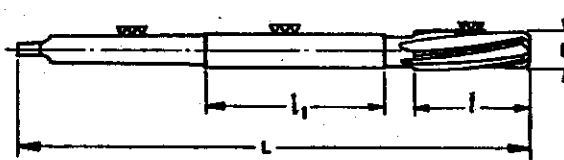
Figure 5.47 Machine jig reamer l_1 . Guide length, l. Cutting edge length, L. Overall length, D. Nominal diameter
